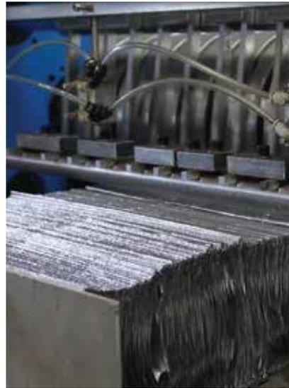
Operations of embossing the aluminum foil and cutting in sheets for the production of embossed foil sheets in various dimensions
