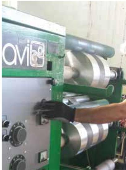
Mother roll cutting operations for the adjustments and dimensions of the final product to meet each unique request
